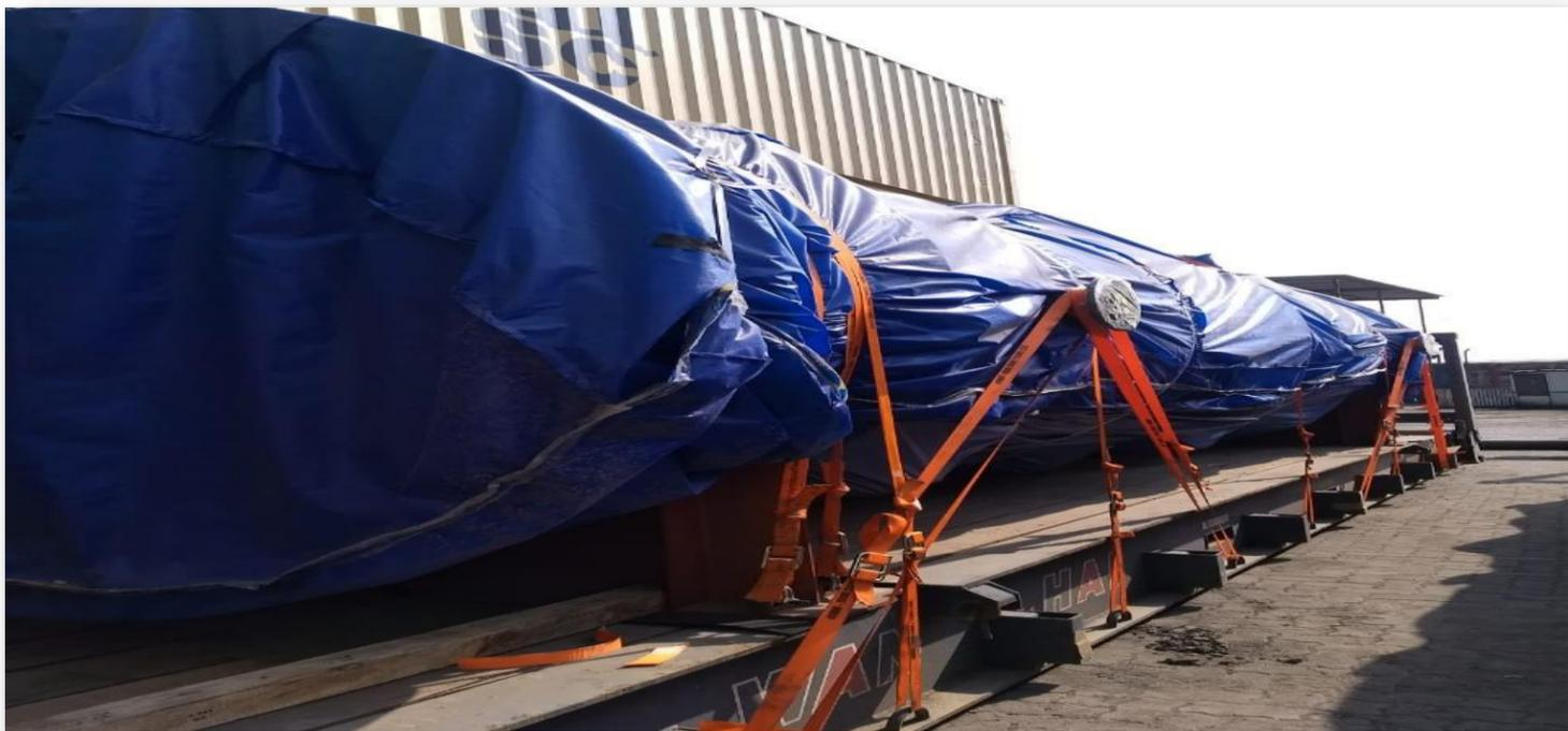
Pressure Vessel with critical timeline delivery, Single piece **29 MT with 11.2 x 2.6 x 2.5 (L x W x H) In Meters** from Nhava Sheva to Cebu, Philippines
